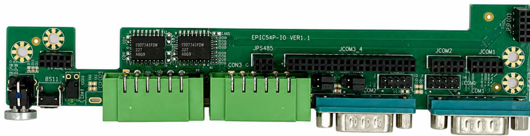
EPIC54P-IO-4CNP VER1.1 GPIO/COM Isolation
